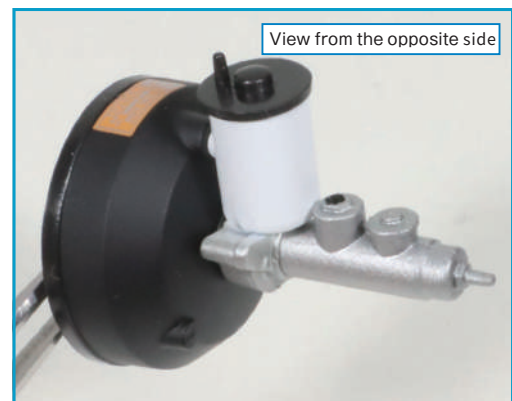
Fit the protrusions of 35-J into the notch and the two screw holes on the reverse side of the 35-K Brake Booster (2) .
